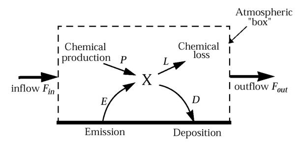
F<sub>in</sub>, F<sub>out</sub>, E, D, P and L together describe the change in the mass of X
