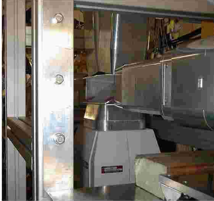
Figure 3.5: Photo of the final focal plane of the separator. The aluminum Z-shaped catcher of thickness 4-6 mm is surrounded by Ge clover detectors.
